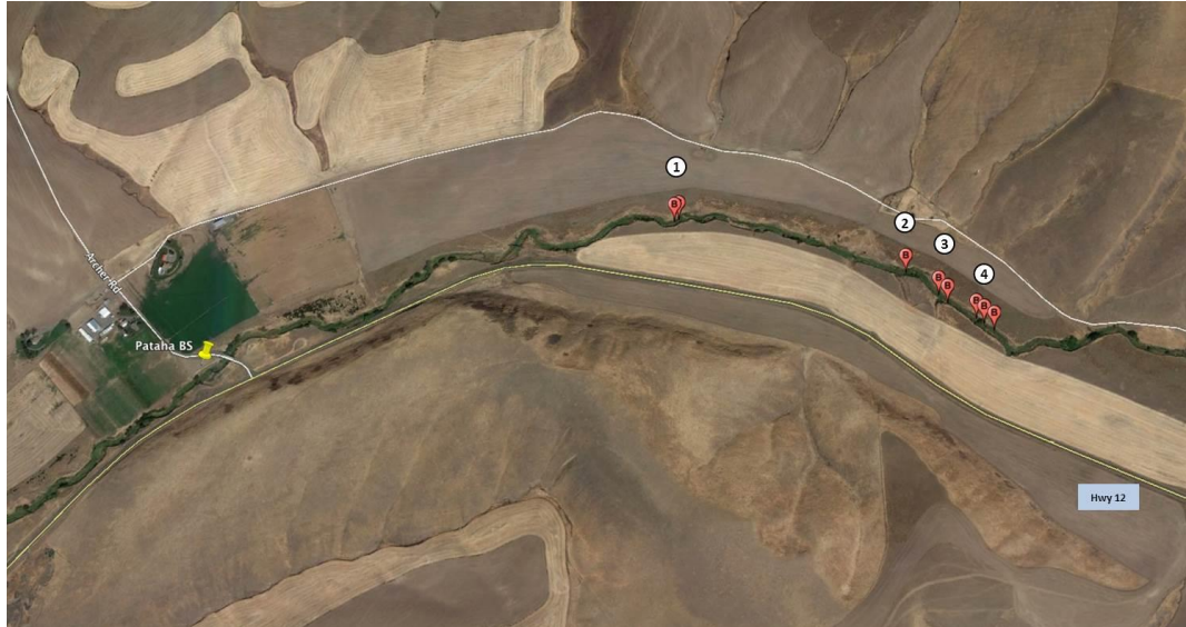
Figure 5. Location of three beaver dam analog complexes and eight total beaver dam analogs (BDAs) along Pataha Creek on the Archer property. “B” = location of individual BDAs, numbers indicate BDA complexes (groups of \geq 1 BDAs designed to function as a group), Pataha BS = bottom of study area.
