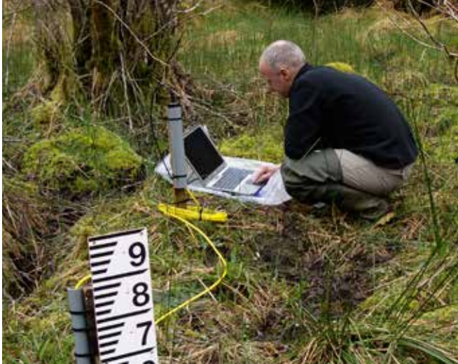
Fig 12. Hydrology monitoring at Knapdale. Automatic loggers and stage boards were used.
