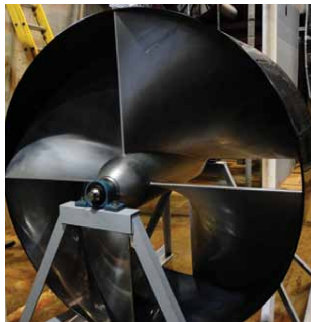
Welka UPG hydrokinetic turbine installed in the Alden flume and evaluated with rainbow trout and largemouth bass. Photo credit: Alden Research Laboratory, Inc.
