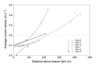
Figure 4. The relationship between average current velocity ( $V_{AVE}$ ) in a beaver pond and the distance above the dam for reach PC. The lines represent linear and exponential models used to estimate the distance ( $K_T$ ) at which  $V_{AVE} = 0.2$  m s<sup>-1</sup>, the threshold velocity separating lentic and lotic habitat (horizontal dashed line).
