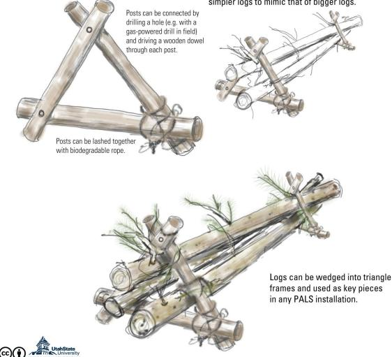
Figure 29 – Smaller logs can be effectively combined into bigger pieces with simple triangular frames. Frames can be sized to hold the smaller logs together, and connected with simple wooden dowels or, biodegradable rope lashing the frame and logs together. These structures can be especially useful where posts cannot be driven into the streambed due to bedrock or compaction.
