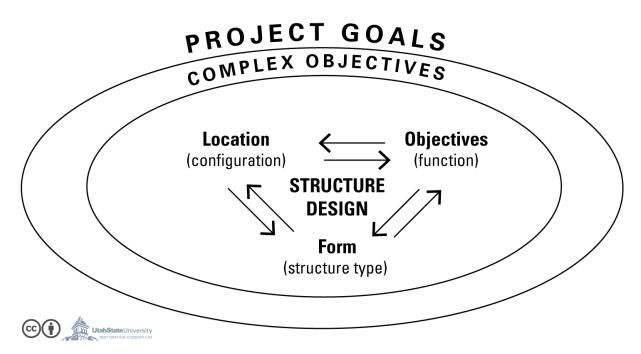
Figure 14 - Structure design is informed by relative location, (i.e., structure configuration within a complex), structure objectives (the function) and form (structure type, size, shape).
