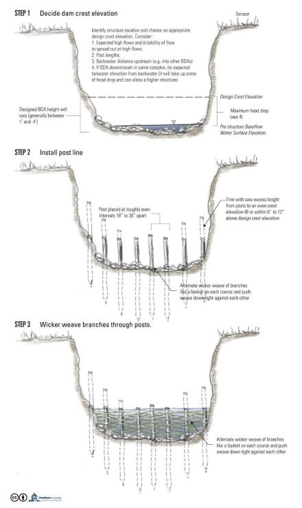
Figure 37 – Typical construction sequence for a post-line wicker weave BDA. First, a single row of posts is installed, and then the wicker weave is placed, and then an attempt is made to patch up the leaks.
