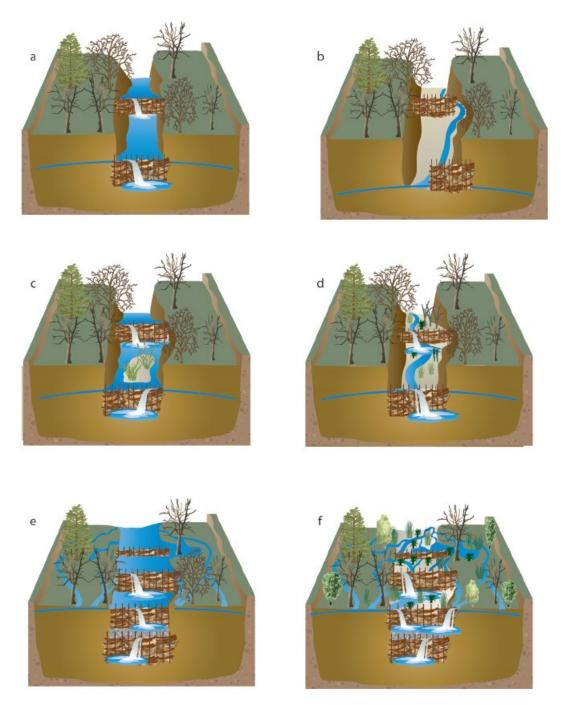
Figure 13 – Expected geomorphic responses following the Cluer and Thorne (2013) channel evolution model (from Stage 3 to 0) after the installation (a) of BDAs, their initial 'failure' by end-cutting (b), subsequent repair (c) and aggradation leading to floodplain reconnection in an incised system. Figure from Pollock et al. (2014). In practice, PALS can force the same processes of channel-widening and aggradation as BDAs.
