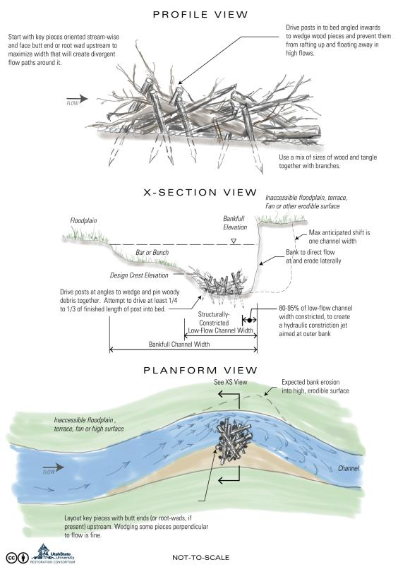
Figure 24 – Typical schematic sketches of a bank-attached PALS intended to blast and erode a bank to recruit sediment and/or wood.
