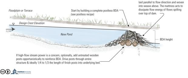
Figure 35 – Profile schematic of post-assisted BDA with key pieces. If you think you need posts, our preferred approach is to build a postless BDA as per Figure 33, and then reinforce after the fact with some posts driven through the structure.
