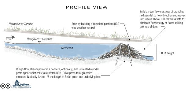
Figure 34 - Profile schematic of post-assisted BDA. If you think you need posts, our preferred approach is to build a postless BDA as per Figure 31, and then reinforce after the fact with some posts driven through the structure.
