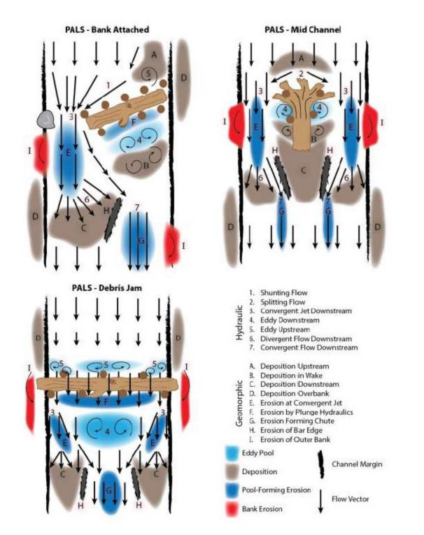
Figure 10 - Hypothesized hydraulic and geomorphic responses associated with bank-attached, mid-channel, and debris jam post-assisted log structures (PALS) from Figure 3.5 from Camp (2015a). Note: what is labeled as 'debris-jam' is referred to in this chapter as 'channel-spanning'.
