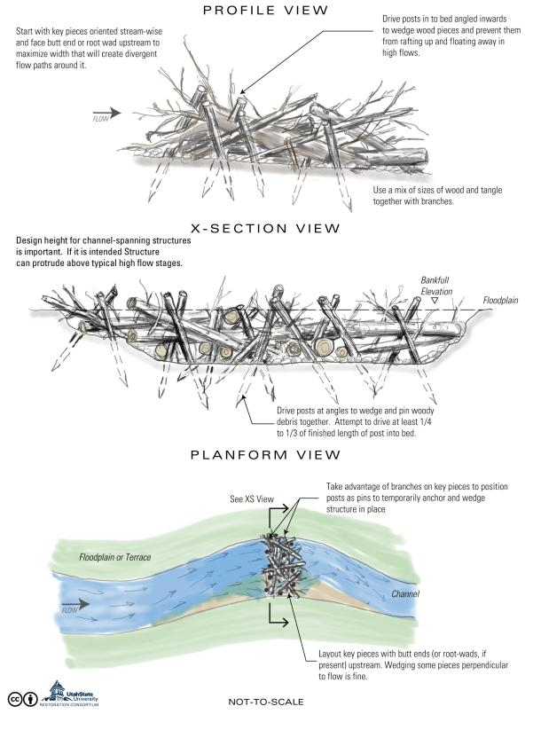
Figure 26 - Typical schematics of a channel-spanning PALS.
