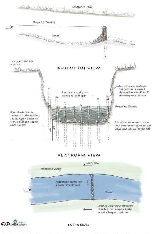
Figure 36 – Typical schematics of the first generation of wicker-weave post-assisted BDAs (similar to Figure 20) using a single row of posts and essentially building a vertical wall. We do not recommend this method, as the wall results in an overflow scour pool that can undermine the base, but in situations where the bed can aggrade quickly in the pond, the deposit can act to stabilize the dam.
