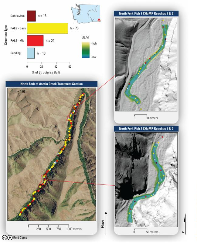
Figure 2 – An example of typical density of structure placement shown at the reach scale (upper and lower right) and at the riverscape scale in lower left. Not only are a high number of structures built, a diverse mix of structure types are used to achieve complex-level objectives (see Chapter 5 for design: Shahverdian et al., 2019b) Figure adapted from Camp (2015a).
