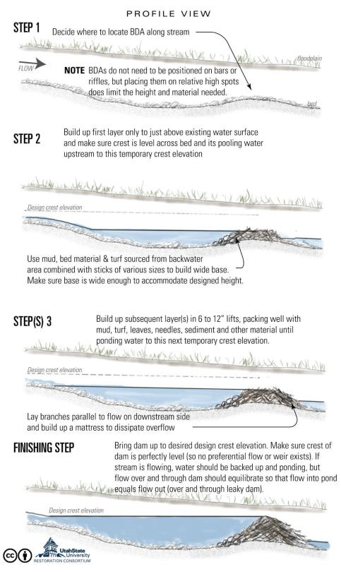
Figure 31 – Sequence for building postless BDAs, build up in 6" to 12" lifts, slowly, like beaver do. Make sure that your lifts are level, and water is backed up sufficiently that is flowing over the crest evenly (as opposed to through or under the dam), and the base is broad, before building up to your next layer.
