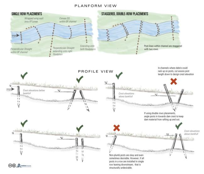
Figure 40 – Post placement considerations. When post are used in BDAs, consideration should be given to whether single-row or staggered double-row placements are used.
