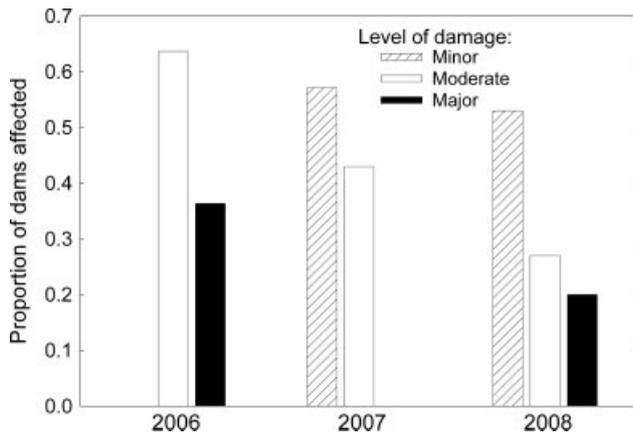
Figure 6. Proportions of monitored dams in each of three damage classes following the spring flood pulses on the BWR. Major damage includes breaches  $>3$ -m wide. Moderate damage includes all breaches  $<3$ -m wide. Minor damage includes loss of some dam component materials and increased leakiness, but little loss of dam functionality. Sample sizes were 11, 7, and 86 for 2006, 2007, and 2008, respectively.
