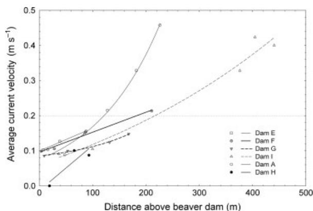
Figure 4. The relationship between average current velocity ( $V_{AVE}$ ) in a beaver pond and the distance above the dam for reach PC. The lines represent linear and exponential models used to estimate the distance ( $K_T$ ) at which  $V_{AVE} = 0.2 \text{ m s}^{-1}$ , the threshold velocity separating lentic and lotic habitat (horizontal dashed line).
