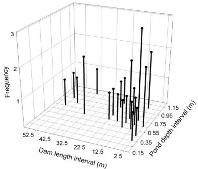
Figure 5. Bivariate frequency distribution for dam size variables  $D_{MAX}$  (maximum impoundment depth near the dam, grouped in 0.1-m intervals) and  $L$  (dam length along crest, grouped in 5-m intervals) for 27 dam/pond complexes examined along the Bill Williams River prior to the 2008 experimental flood. Frequencies are plotted at midpoint value for each interval.
